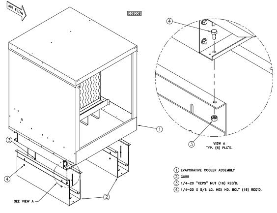
EVAPORATIVE COOLER CURB/PLATFORM MOUNTING ASSY 7-21-03
